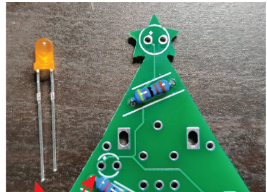
Positive (Anode) Long leg, small + on PCB
