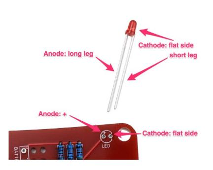
The LED's cathode (-) is indicated by a shorter leg and a flat side of the body, and the anode (+) has a longer leg.
