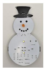
Solder two 3mm white "button" LEDs, and one 5mm orange "carrot" LED.
