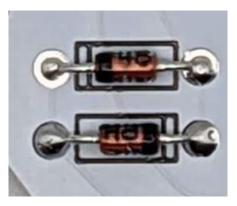
Diodes must be oriented correctly. The side with the stripe is the cathode (-) and the other side is the anode (+).
