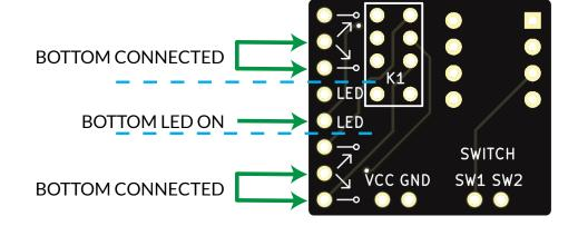
In the other, the middle pad of each pole will be connected to the top pad, and the top LED will be on.
