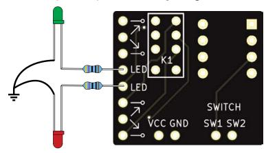
The anode (+) side of the LEDs connects through a resistor to the LED pad on the PCB.
